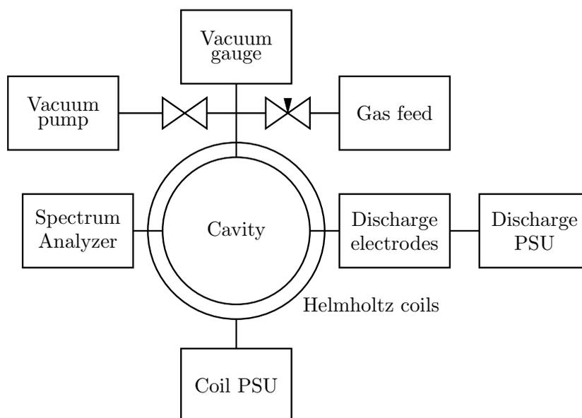
**Figure 2.** Block diagram of the experimental setup. The coils PSU can deliver up to 14 A (20 mT). The vacuum system combined with the gas injection allows for the pressure range from 1 to 300 Pa. The spectrum analyzer also acts as the microwave source for measuring the transmittance of the resonant cavity.
