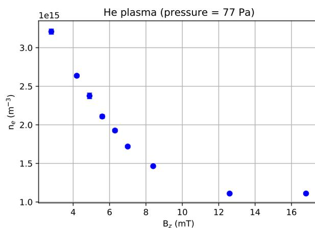
**Figure 8.** Electron density as a function of magnetic field for a helium plasma at the background pressure of 77 Pa.
