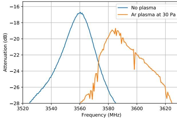
**Figure 6.** Detail of the transmitted power spectrum for an argon plasma at 30 Pa (orange) and without plasma (blue) - discharge switched off.
