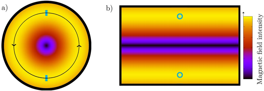
**Figure 1.** Transverse (a) and side (b) views of the magnetic field intensity of the  $TM_{010}$  mode in a cylindrical cavity. The electric field is axial and the magnetic field is azimuthal. The configuration of the loop antennas used to measure the transmittance of the cavity is in blue. The antennas are placed near the region of maximum intensity of the magnetic field; the black line in a) indicates this region.
