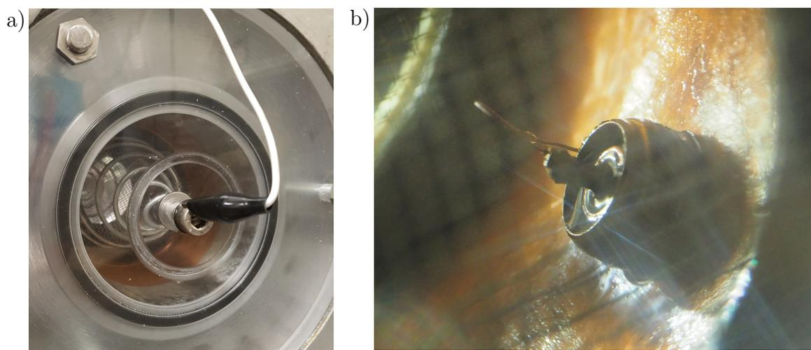
**Figure 3.** a) Cavity top view with the power-source connected to the spring which presses on the aluminum grid. b) Loop antenna used to excite the cavity as illustrated in figure 1. The antenna is soldered to a BNC connector.
