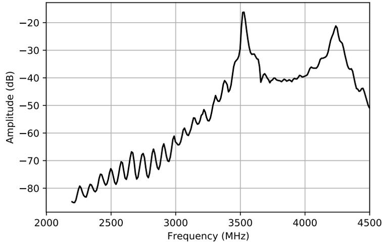
**Figure 5.** Transmitted power collected on the receiving loop as a function of frequency. The first resonant peak is clearly visible at 3.55 GHz with the chamber filled by a helium plasma at 45 Pa background pressure.
