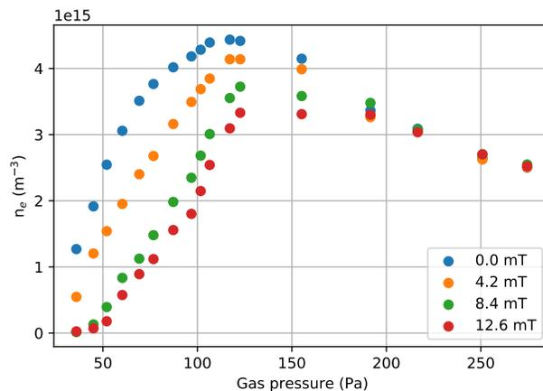
**Figure 9.** Electron densities for a helium plasma as a function of background pressure for different magnetic fields.
