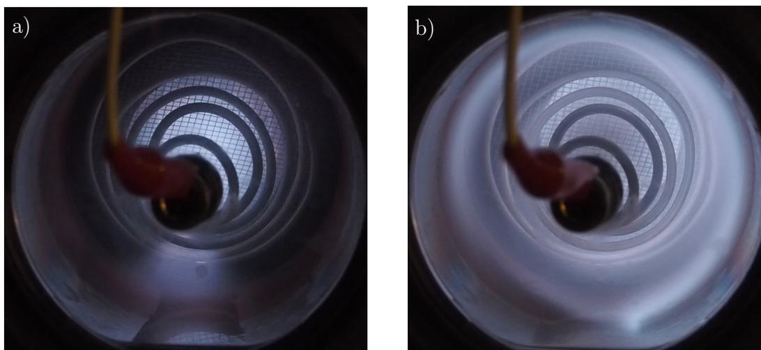
**Figure 10.** Plasma snapshot showing the plasma inside the cavity with: a) no external magnetic field; b) external field of  $\approx 20$  mT. In the presence of the magnetic field, the plasma is pinched in the center of the cavity and expands outwards crossing the metallic grid and coming outside of the electromagnetic cavity to the magnetic confinement.
