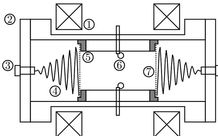
**Figure 4.** Side view diagram of the resonant cavity setup. 1 - Helmholtz coils; 2 - Acrylic window; 3 - Discharge electrode; 4 - Coil spring; 5 - Mesh insulator; 6 - Antenna; 7 - Aluminum mesh
