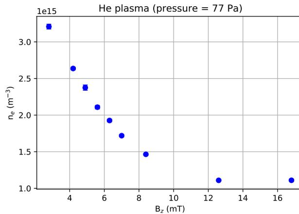
**Figure 8.** Electron density as a function of magnetic field for a helium plasma at the background pressure of 77 Pa.
