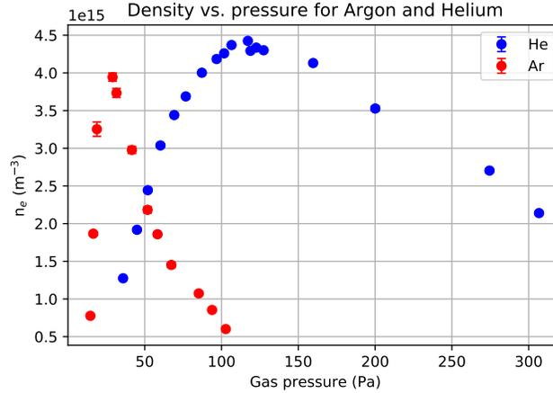
**Figure 7.** Electron density as a function of background pressure for both helium and argon plasmas.
